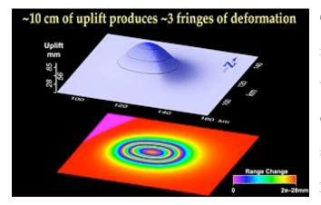
enough to sense change as small as 0.00006 of a degree.<sup>9</sup> Another method which is becoming more widely used to measure all aspects of ground deformation is called satellite radar inferometry. This process utilizes radar signals sent
